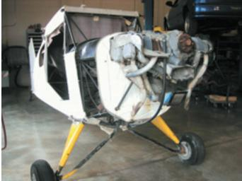
completed, an inspector came in to decide whether it was at all possible to restore its airworthiness. It was approved. Finally, the class documented the parts: which were in good condition, which were missing, and which needed repair.
